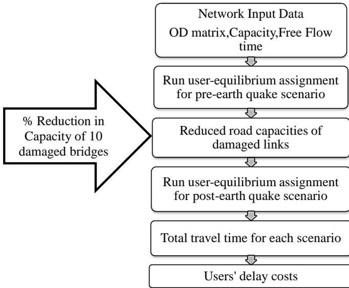
Figure 6. Methodology flow chart for delay estimation.
